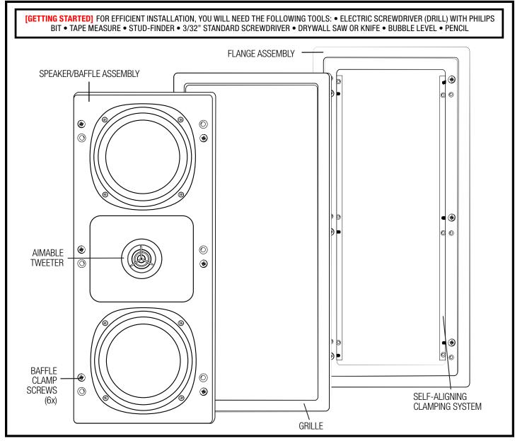
Thank you for purchasing the Phase Technology® CI110 II high definition in-wall speaker system. The mounting frame of extruded aluminum has a uniquely designed self-aligning clamping system to secure the flange assembly to the drywall. This patent pending design simplifies installation and reduces unwanted wall vibration resulting in improved performance and definition.
