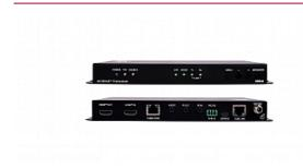
KDS-8 is a high-performance, zero latency, 4K@60Hz (4:4:4) video streaming transceiver for streaming via Ethernet over copper cable. KDS-8 can be set as either an encoder or decoder. As an encoder, it encodes and streams the HDMI input along with IR, RS-232, and analog audio, over an IP network. As a decoder, it receives the encoded signal and decodes it for output
