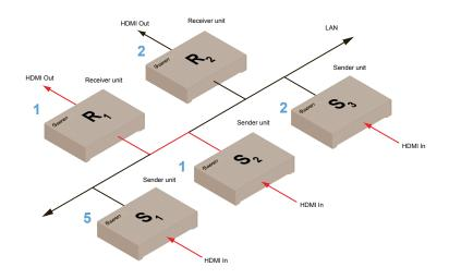
Figure 2.5 - Unicast mode: Sender S2 transmitting to Receiver unit R1.
