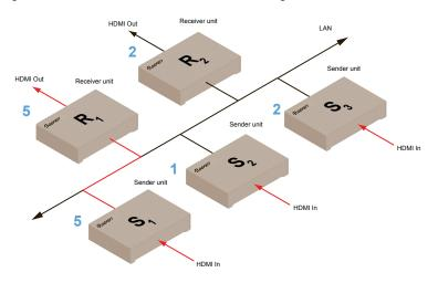
Figure 2.6 - Unicast mode: Sender unit S1 transmitting to Receiver unit R1
