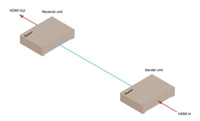
Figure 2.3 - DHCP or Static IP mode: A Sender and Receiver unit connected to a network (LAN).
