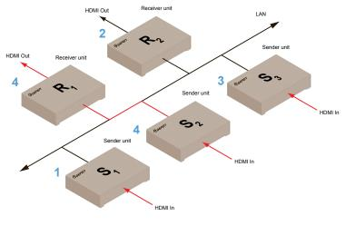
Figure 2.1 - Switching between Sender units (sources).
