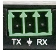
This is how the cable should look. If using the AC-CABLE-3.5-DB9F (Female) or AC-CABLE-3.5-DB9M (Male), the colors will be the same. With any other cable, please follow Tx, G, Rx as shown above. A RS-232 cable preparation diagram is on the next page.
