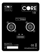
All Core Speaker Cabinets use a four-pole Twist-lock input jacks wired for 1+ to the Positive speaker lead and 1- to the Negative speaker lead.
