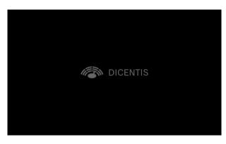
When the DCNM-MMD cannot find the system in the network, the following screen is shown. Refer to **Installation Test** in the "Hardware Installation Manual".
