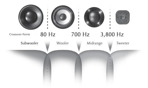
Above: The S4X crossover routes audio signal to their intended drivers at specific frequencies (700 Hz, 3,800 Hz). Because the S4X produces such a steep crossover slope, Induction Dynamics is able to use the best possible drivers for each frequency range. Subwoofer crossover points are generally selectable through your subwoofer amplifier. Induction Dynamics recommends a subwoofer crossover point between 50 - 60 Hz.
