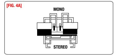
**STEREO FIG. 4A**-8 ohms: Use this configuration to drive one channel (left OR right) of a stereo pair. Set jumper plugs in the stereo position. (Fig. 4A) Connect the right or left signal wire to the right set of terminals on the rear of the speaker. Leave the front panel switch left signal wires to the spring-loaded in the Bipole position.
