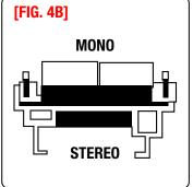
MONO/STEREO FIG. 4B-4 ohms: Use this configuration to drive one channel (left OR right) of a stereo pair with a 4 ohm speaker load. Set jumper plugs in the mono position. (Fig. 4B) Connect the right or left signal wire to the left set of posts on the rear of the speaker. Acoustic output of the speaker is increased by 3 dB in this configuration.
