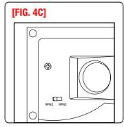
BIPOLE/DIPOLE FIG. 4C-4 Use this configuration for home theater surround applications. For bipole mode, connect as in the Mono/Stereo instructions (FIG. 4C): one speaker to each surround channel. For dipole mode, connect speaker inputs the same as Mono/Stereo instructions (FIG. 4C). but reverse the + and - connections of the red and black tweeter wires to put one of the tweeters out of phase.
