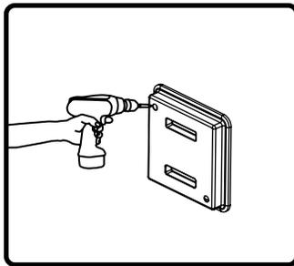
5. Insert speaker into mounting hole with paint mask in place. Tighten both screws on the baffle face to actuate the mounting wings. Firmly secure both screws. **DO NOT OVERTIGHTEN.**
