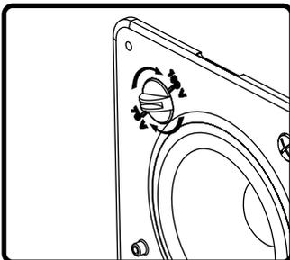
9. Adjust tap switch to proper setting. Switch is preset to 8 Ohm mode.
