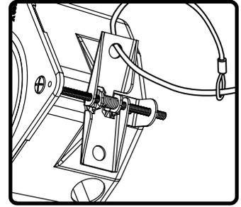
4. If required, attach seismic restraint system to hole in clamping arm, then to reinforced structure (saftey cable not included)
