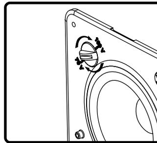
7. Adjust tap switch to proper setting. Switch is preset to 8 Ohm mode.
