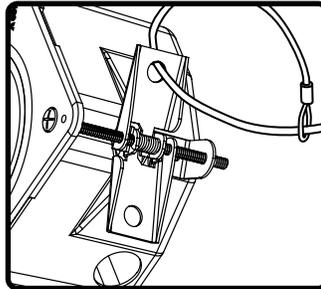
6. If required, attach seismic restraint system to hole in clamping arm, then to reinforced structure (safety cable not included)
