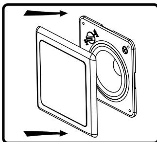
9. Align tabs on snap-fit grille with slots in baffle. Gently press grille into place.
