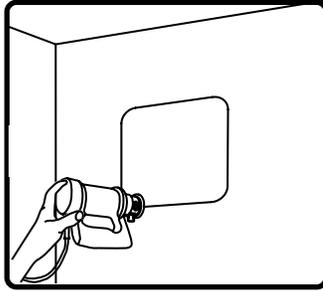
2. Use hole template to mark cutout on sheetrock. Use RotoZip or other tool to cut hole. Hole size: 4" (102 mm) H x 4" (102mm) W.
