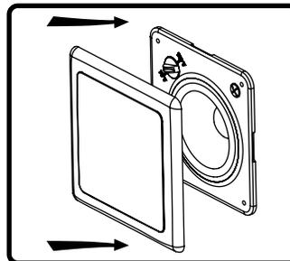
11. Align tabs on snap-fit grille with slots in baffle. Gently press grille into place.
