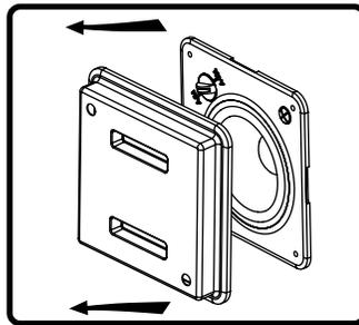
6. Remove paint mask unless painting is required. In that case, follow steps 7-10 when painting is complete.
