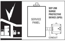
For use before or after the main disconnect for optimum lightning protection.
