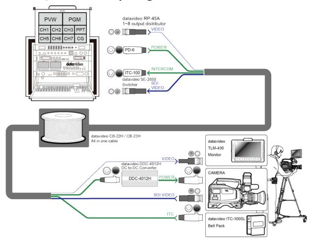
**Note:** PIN definition of the CB-22H/CB-23H Power Cable should match that of the PD-6 Power Center. The purpose is to prevent the camera from being damaged by high voltage power. The CB-22H/23H must be used with the PD-6.
