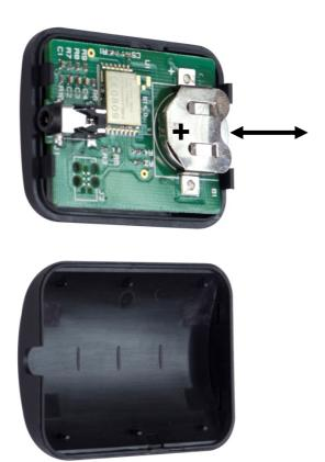
This button battery can be replaced by the user when it dies. **Please remove the case back carefully** to avoid user damage to the PCB or case. Then slide the old battery out.
