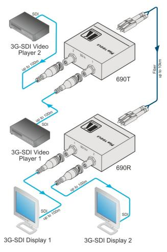
Figure 3: Connecting the 690T and/or 690R
