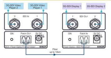
The SDI 1 IN source signal on the 690T is always routed to the SDI 1 OUT acceptor on the 690R and the SDI 2 IN source signal on the 690T is always passed to the SDI 2 OUT acceptor on the 690R
