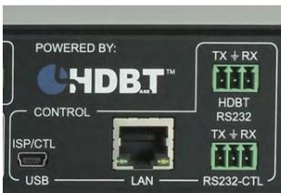
To do Advanced Routing, send RS232 signals here
