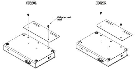
2. Screw the bracket into any convenient location on the rack.
