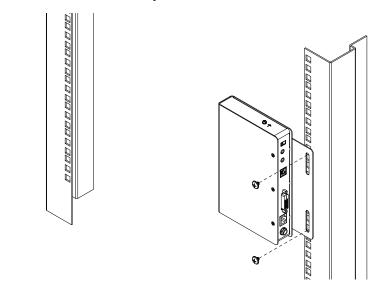
**Note:** These screws are not provided. We recommend that you use M5 x 12 Phillips Type I cross, recessed type screws.
