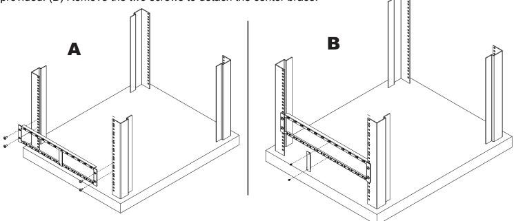
2. Place the video extender on the 2U Mounting Plate and align the holes, then screw the video extender to the mounting plate.
