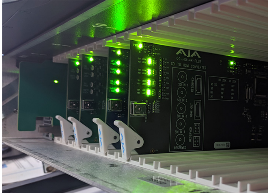
Figure 8. The white plastic tab for the card second from the right is now upright. All cards are shown fully inserted.
