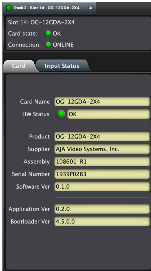
Figure 10. OG-12GDA-2x4 Card Tab Screen in Dashboard
