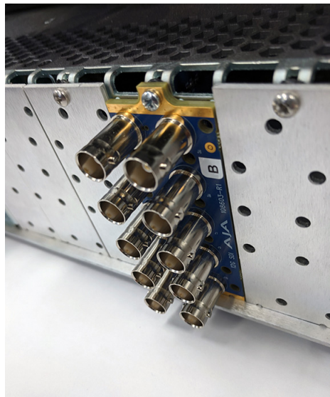
Figure 6. Rear Card Inserted Into Frame Seating Slot
