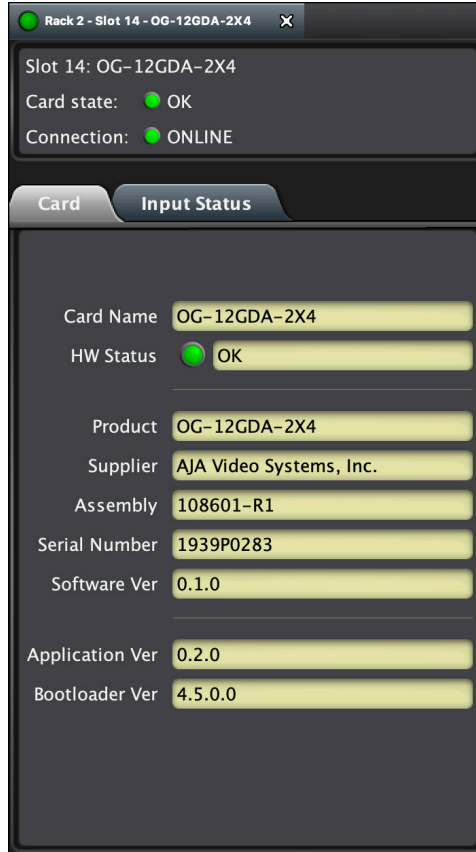
Figure 15. OG-12GDA-2x4 Card Tab Screen in DashBoard indicating the currently installed software version.
