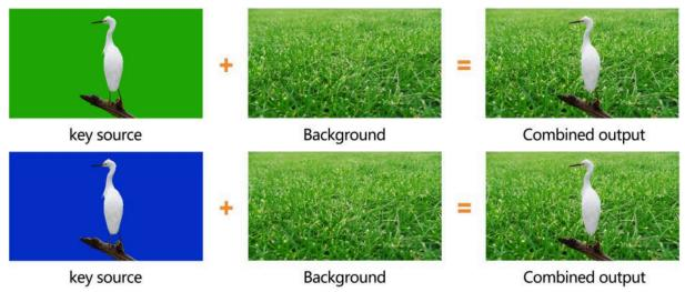
Press the CHROMA Key button, press the Menu knob and choose Chroma to configure the effect of Chroma Key, including the Key Source, Key Color, Clip, Gain, Key Fetch, Mask, etc., detailed parameters setting as below.
