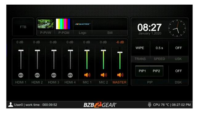
The taskbar below shows username, working time, USB connection, CPU working temperature, and system time in the bottom of the Status/Menu page.
