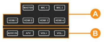
Part A: Used for selecting one audio source to be configured, including Master, MIC 1, MIC 2, HDMI 1, HDMI 2, HDMI 3, and HDMI 4.
