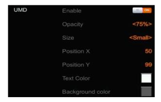
The UMD text content for the 4 HDMI inputs can be set from the menu. Users can rename the UMD content for each window by using a virtual keyboard and rotary button. It supports up to a maximum of 10 characters for each input. In the example below the input has been renamed from HDMI 1 to CAM1.
