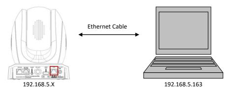
On your PC/laptop, open a web browser and in the address bar, enter the camera's default IP address, 192.168.5.163 then press the **ENTER** key which should take you to login page of the web interface.
