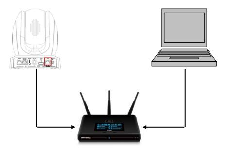
In order to enable the camera's DHCP mode, simply check the DHCP checkbox to allow the router to dynamically assign an IP address to PTC-140NDI.
