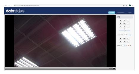
Stream At the bottom right corner of the camera image display window, click the "Stream" button to switch between Main Stream and Sub Stream previews. See **Video Encode** in **Configuration** tab for stream settings.
