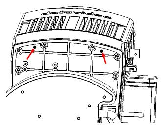
2. Use the two M3 screws that come with the product package to secure PCB-1 to the position as indicated by the arrows in the diagram below.
