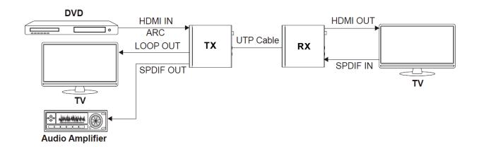
**Example 3:** Set the extender to ARC mode, then toggle the LOOP-OUT/ AUDIO ONLY switch to the right. The HDMI OUT port of the transmitter is now set to AUDIO ONLY.
