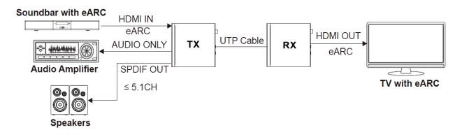
**Example 6:** Set the extender to eARC mode, then toggle the LOOP-OUT/ AUDIO ONLY switch to the left. The HDMI OUT port of the transmitter is now set to LOOP OUT.
