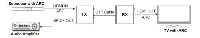
**Example 5:** Set the extender to eARC mode, then toggle the LOOP-OUT/ AUDIO ONLY switch to the right. The HDMI OUT port of the transmitter is now set to AUDIO ONLY.
