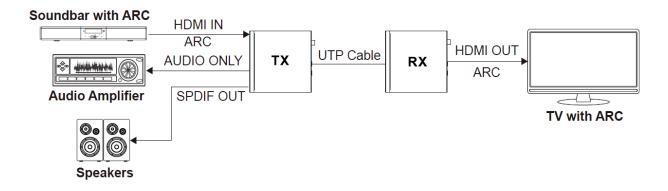
**Example 4:** Set the extender to ARC mode, then toggle the LOOP-OUT/ AUDIO ONLY switch to the left. The HDMI OUT port of the transmitter is now set to LOOP OUT.
