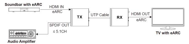
Note: In eARC mode, the SPDIF OUT port can only output the audio up to 5.1CH.
