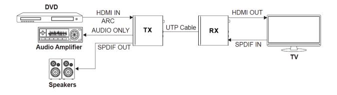
**Example 2:** Set the extender to SPDIF mode, then toggle the LOOP-OUT/ AUDIO ONLY switch to the left. The HDMI OUT port of the transmitter is now set to LOOP-OUT.
