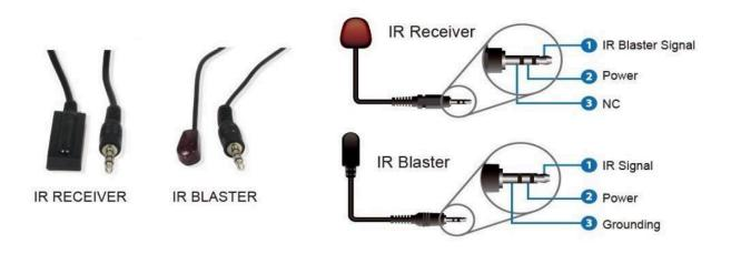
**Note:** When the angle between the IR receiver and the remote control is  $\pm 45^{\circ}$ , the transmission distance is 0-5 meters. When the angle between the IR receiver and the remote control is  $\pm 90^{\circ}$ , the transmission distance is 0-8 meters.
