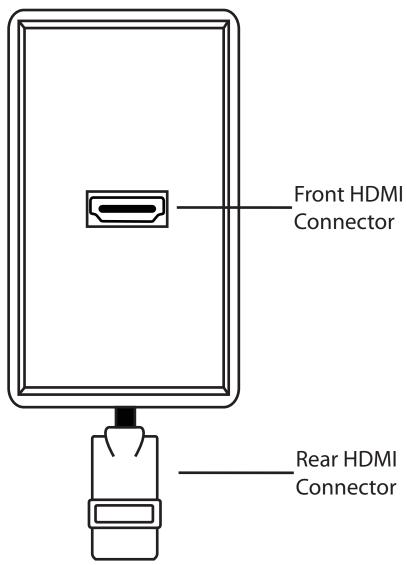
3. Remove the Face plate from the wall plate by pushing down on HDMI connector with your thumbs and at the same time pulling two opposite corners away. Under the face plate you will find two screws hidden there. Place the wall plate against the opening of the electrical box, then thread the two supplied screws through the screw holes in the wall plate and the electrical box, then tighten the screws and reattach the face plate.
