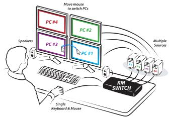
HSL 4-Port KM Switch System Diagram
