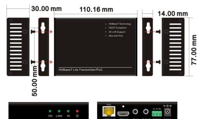
Figure 5-1 Panel drawing of HDMI Twisted Pair PoETransmitter
