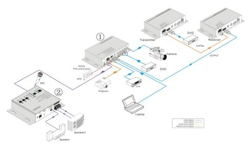
Figure 3-2 Collocation Products Connection Diagram
