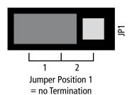
If you want to switch-off the termination, remove carefully the jumper from the two pins of position 2 of the socket and plug it onto the two pins of position 1 (see adjacent sletch).
