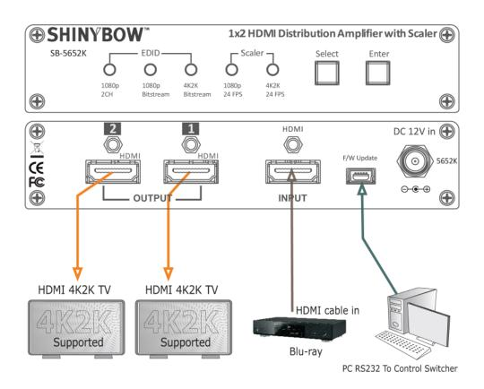
Application use 1080p and 4K2K HDTV via 1x2 Distribution Amplifier with Scaler.
