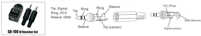
SB-100 Receiver and SB-101 Transmitter The DISTANCE maximum ~ 984 feet (300M)
