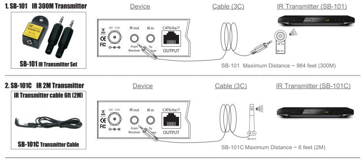
\*\*\* When you plug the External IR extender into the switcher, the front panel IR transmitter remains active. \*\*\*
