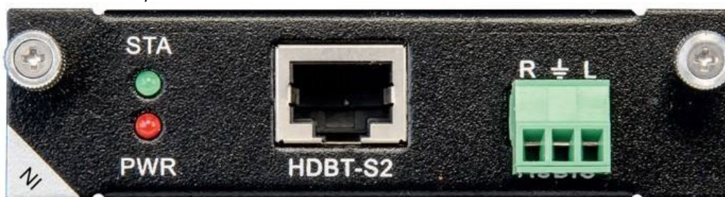
1 Port HDBT input card with analog audio embedding, supports RS232 passthrough.
