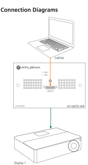
**Note:** This connection will only work with HDBaseT compatible projectors.
