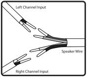
3. Connect the speaker wire to the input signal wire. Each wire bundle has two channels:
