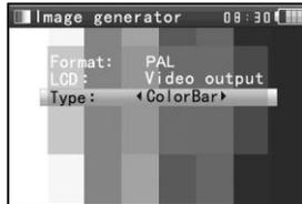
The tester’s color bar generator supports both PAL and NTSC format color bars.
