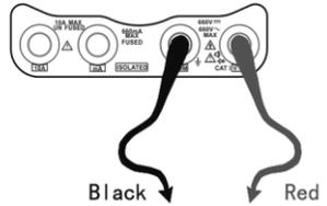
c. Before connecting the test leads across the two sides of the capacitor under measurement, be sure that the capacitor has been fully discharged.
