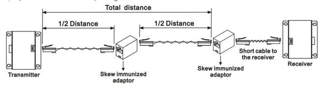
CAUTION: to avoid display equipment damaged, be sure to make correct cable connection and power for both AT-COMP300SL before connecting AT-COMP300RL.
