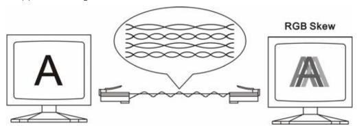
2. Recommend to use following cabling design to reduce skew status, to add special made "skew immunized adaptor", 2 pieces included at the package.
