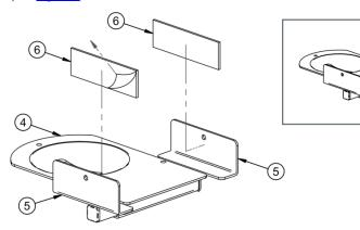
Figure 5: Attaching the Foam Pads
