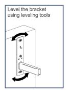
Figure 2: Attaching the Bracket to a Concrete Wall
