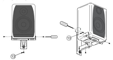
Figure 8: Securing the Speaker
