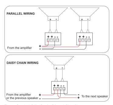
Figure 5: Open-back Ceiling Speaker Schematic Pinout Diagram
