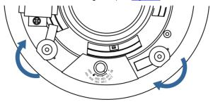
Figure 3: Position Mounting Tab
