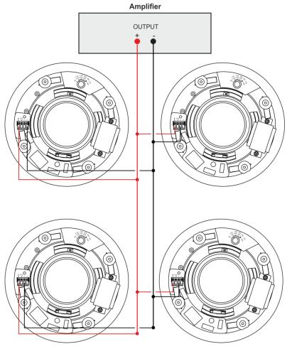
Figure 10: Square Layout Parallel Wiring
