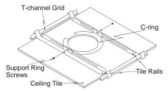
Figure 6: Installing the Open-back Ceiling Speakers
