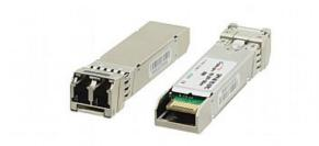
OSPMM1 is a fiber optic transceiver for 850nm multimode signals. This standard pluggable SFP+ optical module has two LC connectors for reception and transmission of signals over two strands of multimode optical fiber
