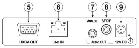
Figure 4: TP-122xl UXGA/Audio Line Receiver Rear Panel
