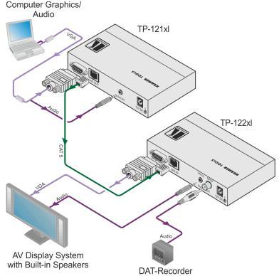
Figure 5: Connecting the TP-121xl Transmitter and TP-122xl Receiver
