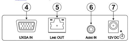
Figure 2: TP-121xl UXGA/Audio Line Transmitter Rear Panel
