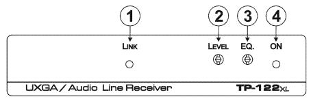
Figure 3: TP-122xl UXGA/Audio Line Receiver Front Panel
