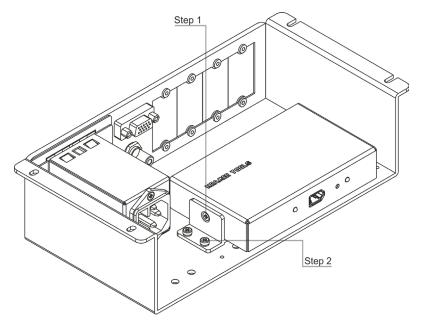
Figure 3: Installing a Kramer TOOL
