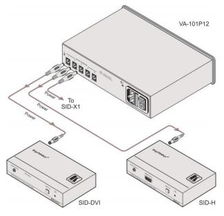
Figure 3: Connecting the VA-101P12, VA-102P12 Description
