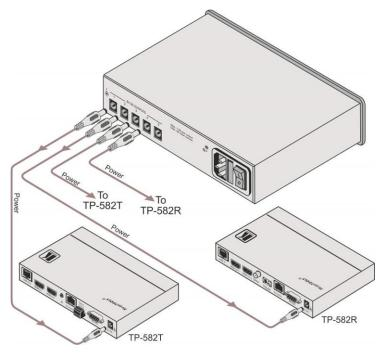
Figure 3: Connecting the VA-101P5 Power Supply
