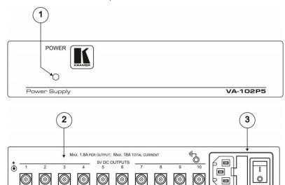
Figure 2: VA-102P5 10-Output 5V DC Power Supply
