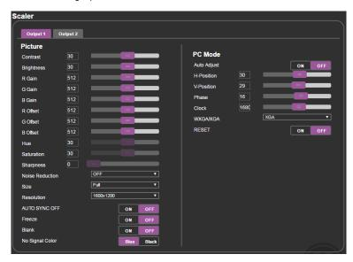
Figure 21: The Scaler Page - Output 1 for an Analog Input
