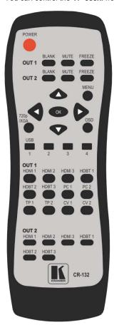
Figure 13: Infrared Remote Control Transmitter
