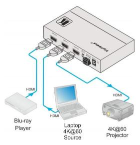
Figure 2: Connecting the VS-211H2 Automatic HDMI Standby Switcher
