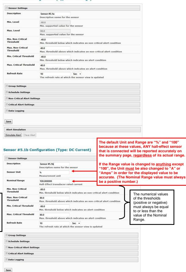
Most of the sensor settings are the same as any other sensor configuration (page 39 of the ENVIROMUX-xD manual) but for the DC Current Sensors there are some differences:
