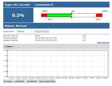
Click on the "Configure" button on any Status Page to display the Configuration page for any sensor.
