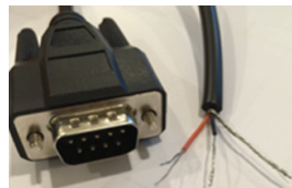
KD-3.5MDB96 after stripping wire
