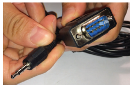
KD-3.5MDB96 with 3.5mm TRS Connector
