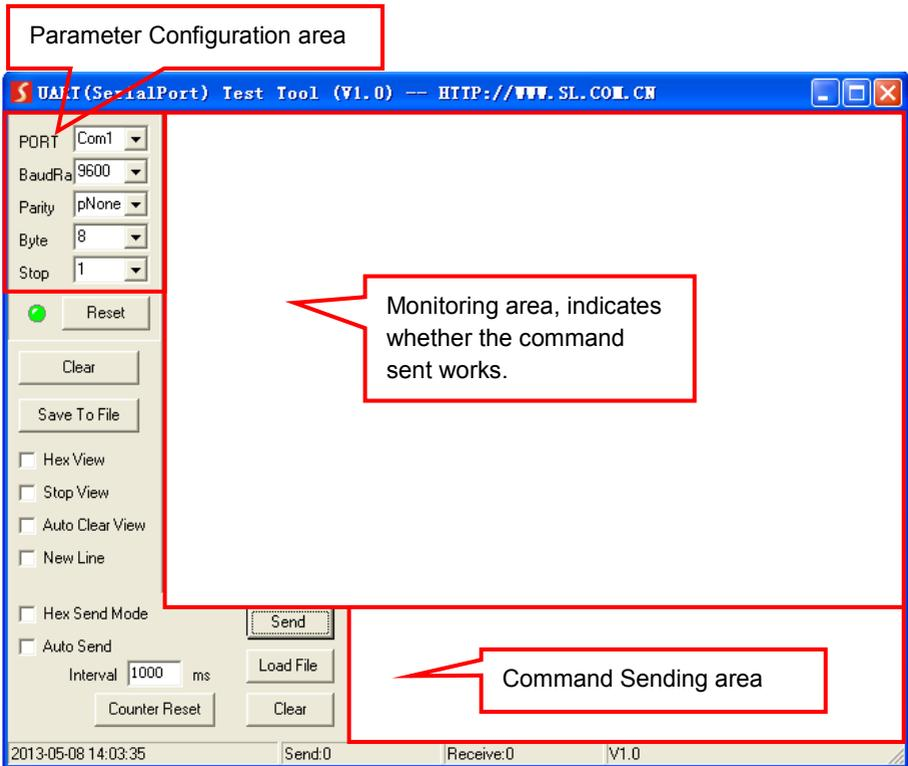
Please set the parameters of COM number, bound rate, data bit, stop bit and the parity bit correctly, only then will you be able to send command in Command Sending Area.
