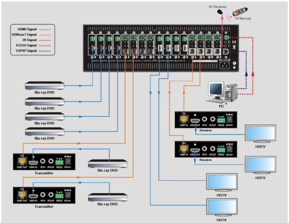
**Figure 3- 1 Connection Diagram**
