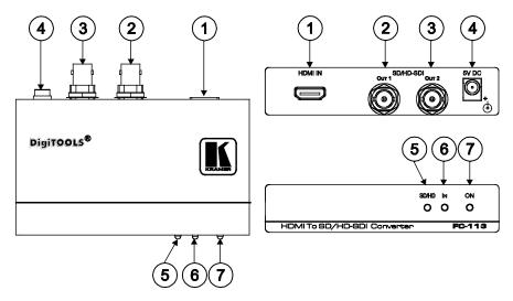
Figure 1: FC-113 HDMI to SD/HD-SDI Converter
