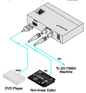
Figure 2: Connecting the FC-113 HDMI to SD/HD-SDI Converter
