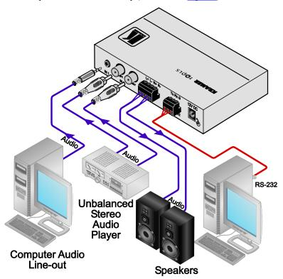
Figure 3: Connecting the 900xl Power Amplifier
