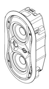
than 4 inch deep providing an easy installation into nearly any tight wall or ceiling space. A rear cover, with provisions for a junction box fitting, provides access to a 4-pin terminal block that allows direct connection to the speaker and provides pass through to additional speakers. FM4.2 loudspeakers provide wide dispersion, high-efficiency, high-maximum output, ease of installation, and wide-range reproduction of music or voice.
