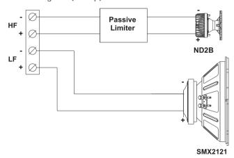
Block Diagram (passive): Standard shipping configuration
