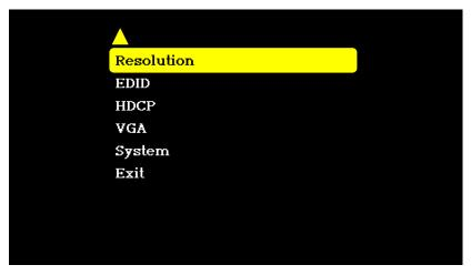
Resolution - Manage the built-in scaler's output resolution. This option affects both the HDMI and VGA inputs.
