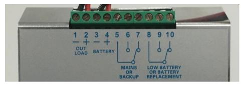
Connect your device to the 48VDC @ 5A power source on Pins 1 and 2.
