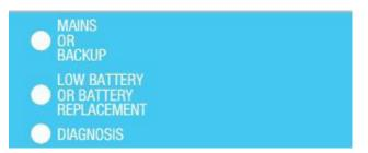
Mains or Backup LED will be off when AC power is available and on when powered by the battery.
